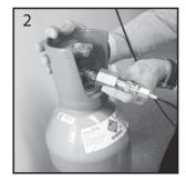
Connect the Tube to the cylinder.
